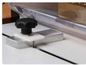
Micro switch is a sensor that will automatically trigger the punch when the paper is inserted into the die slot.For a more efficient workflow.
